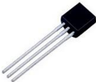
FIG: TEMPERATURE SENSOR
